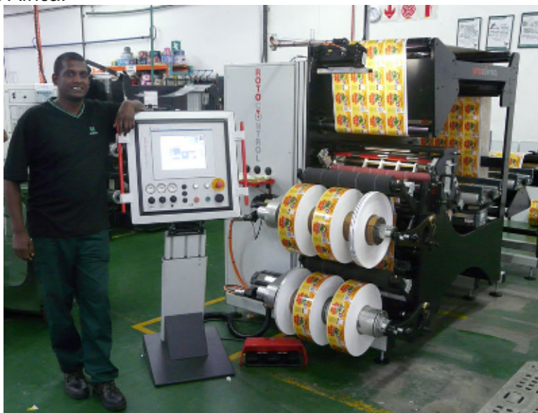
Pictured above: Bashir Mohideen (Uniprint) beside installed ROTOCONTROL RSC slitter/rewinder inspection machine
