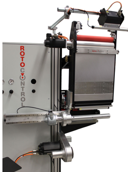
ROTOCONTROL slitter/rewinder inspection machine with vacuum splice table
