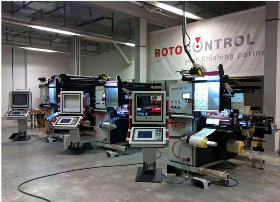
*Three ROTOCONTROL slitter/rewinder inspection machines that shipped to the UK*
