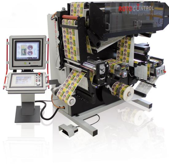
*ROTOCONTROL slit/rewinder inspection machine to be demonstrated at Graficon-GIDUE Open House*
