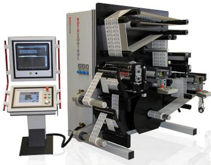
*ROTOCONTROL RSC Slitter/Rewinder Inspection Machine*
