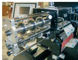
At New Era Labels, RotoControl's cartridge slitting system is allowing fast job changes using either razor or shear knife cartridges.
