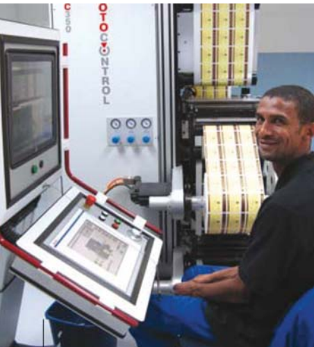
In March this year, SA Litho installed three RSC 340 slitter rewinders, complete with AVT Helios 100% inspection systems.
