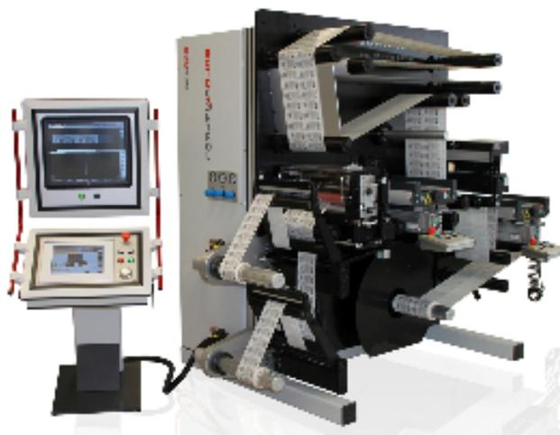
*ROTOCONTROL RSC Slitter/Rewinder Inspection Machine*
