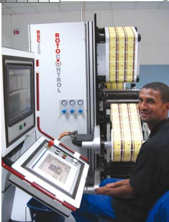
In March this year, SA Litho installed three RotoControl RSC 340 slitter rewinders, complete with AVT Helios 100% inspection systems.
