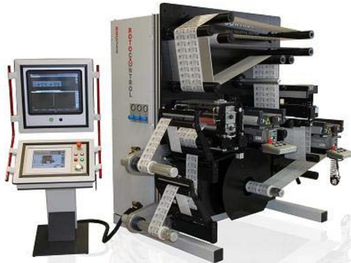
*ROTOCONTROL RSC Slitter/Rewinder Inspection Machine*
