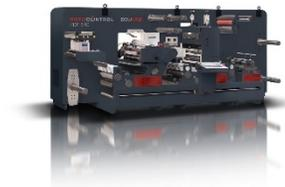
The ROTOCONTROL ECOline RDF converting and finishing system for digitally printed labels
