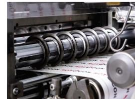
The second upgrade, which has been in big demand from customers requesting a more affordable and efficient format, is a high-speed matrix stripping system. It ensures no web in between the stripping shaft and matrix, preventing waste breakage and machine downtime. Additionally, a servo-driven motor enables ideal stripping tension, even in the presence of matrix coil diameter variations. This avoids any issues caused by special substrates or die-cutting complex label shapes.
