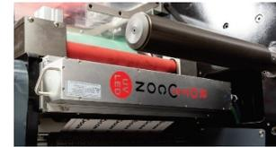
Additionally, the UV LEDs' instant on/off capability means no more waiting to restart the machine after a power outage. Faster changeovers via flexible controls and curing adjustments are also possible – contributing to improved uptime and higher production rates.
