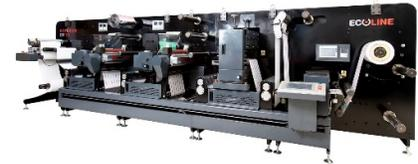
▶ ▶ A first major upgrade of the RDF 330 is an automatic shear knife slitting system that simplifies the normally time-consuming set-up and tweaking required when manually adjusting blades across more than three lanes. The operator can now enter the label sizes, gap sizes, and number of slits then the system will automatically bring all the blades into the right position with the correct gaps.
