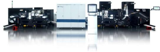
**The ROTOCONTROL DT-340 digital label finishing machine with an integrated Domino N610i label press**
