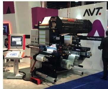
**The ROTOCONTROL RSP-V series pharmaceutical finishing machine with the AVT Helios II automatic 100% print inspection solution**
