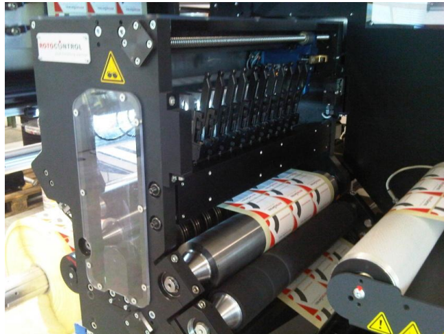
Die neue ROTOCONTROL EPOS Option (Electronic Knife Positioning System)
